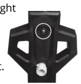
4 Slide the roller holster onto the middle of the roller handle bar and screw into the bar.
