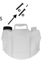
2 Attach each metal loop on the backpack straps to the bottom two loops on the tank.
